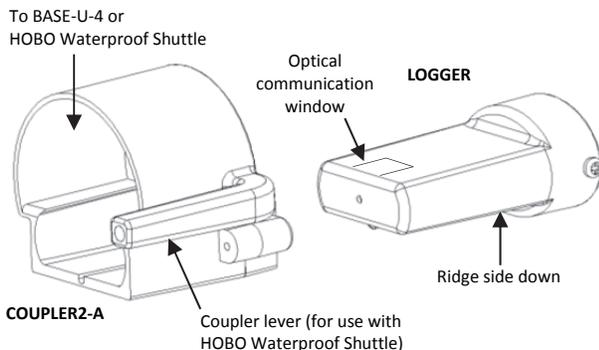
3. If you are using the HOBO Waterproof Shuttle, briefly press the coupler lever to put the shuttle into base station mode.
