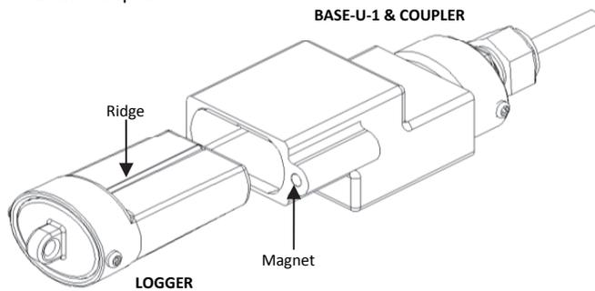
For BASE-U-4 or the HOBO Waterproof Shuttle, firmly insert the optical end of the base station into the D-shaped end of the coupler, and make sure that the ridge on the logger is aligned with the groove in the coupler.
