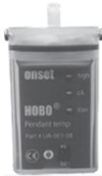
The HOBO Pendant Temperature Data Logger is a waterproof, one-channel logger with 10-bit resolution and can record up to approximately 6,500 (8K model) or 52,000 (64K model) measurements or internal logger events. The logger uses a coupler and optical base station with USB interface for launching and data readout by a computer.
