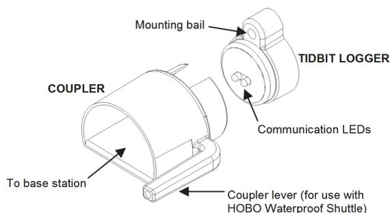
When properly seated, the logger should be nearly flush with the top of the coupler.
