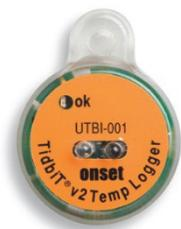
The Tidbit v2 Temp logger is Onset's smallest U-Series logger. Its durable, waterproof case is designed for extended deployments measuring temperature in streams, lakes, oceans, coastal habitats, and soils. The logger's small size allows it to be easily mounted and/or hidden in the field. It is waterproof up to 305 m (1000 feet) and rugged enough to withstand years of use. It has enough memory to record over 42,000 12-bit temperature measurements.
